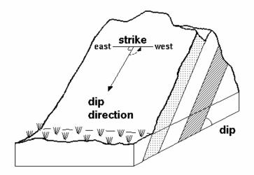
**STRIKE** - The bearing of the line of intersection of plane and horizontal plane is called strike. Bearing is the horizontal angle between a line and a specified coordinate direction, usually true north.
